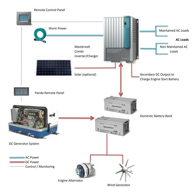
DC Hybrid Power System - using Mastervolt Combi with built in changeover switch, MPPT Solar regulator. Two AC inputs and two AC outputs allow for maintained and non-maintained AC loads.
