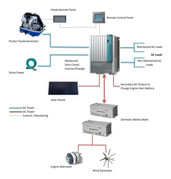
AC Hybrid Power System - using new Mastervolt Ultra Combi with built in changeover switch, MPPT Solar regulator. Two AC inputs and two AC outputs allow for maintained and non-maintained AC loads. Auto start of AC generator as and when load requires.
